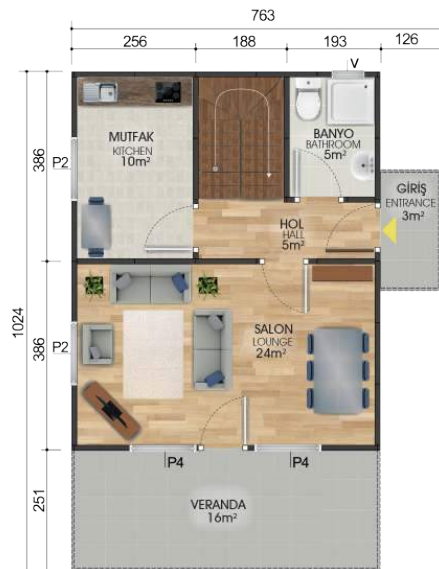
Zemin Kat Planı / Ground Floor Plan 49m 2 + 19m 2 = 68m 2
