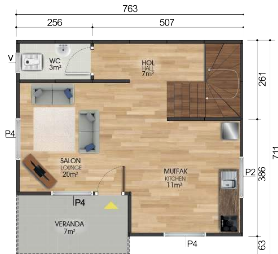
Zemin Kat Planı / Ground Floor Plan 45m 2 + 7m 2 = 52m 2
