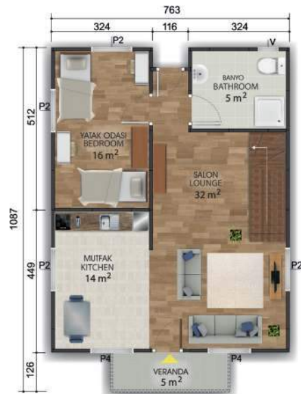
Zemin Kat Planı / Ground Floor Plan 74m 2 + 5m 2 = 79m 2
