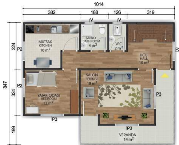
Zemin Kat Planı / Ground Floor Plan 64m 2 + 14m 2 = 78m 2
